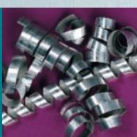
Precision Rod's short, tight and compact chips from form tools allow machinery to operate smoothly, minimizing downtime and costs. Whereas competitive grades' chips are typically long, stringy spirals that often entangle with themselves and machine tools, causing unwanted disruptions to clear the chips.
